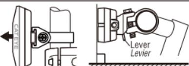
Securely attach the light and the reflector has to be perpendicular to the ground.
