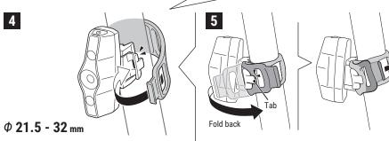
Attach the light securely in the mounting position.
