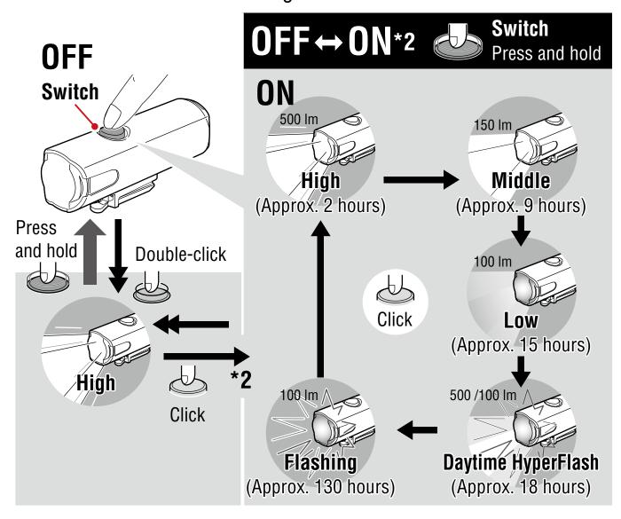
\*2 When turning the light on, it lights up in the mode that was used last time. (Mode memory function)
