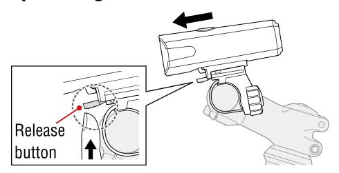
\* To readjust the beam angle, loosen the dial and/or the screw enough to move the bracket, and firmly tighten them after adjustment.
