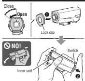
How to remove Rubber gasket hatteries Press the lens side of the upper battery.
