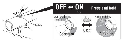
\*1 When you turn the light on, it lights up in the last lighting mode you used. (Mode memory function) When the switch (indicator) lights up, the remaining battery power is 20% or less. Please charge as soon as possible.
