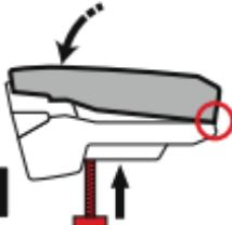
Remove top body by pushing while sliding it backward.
