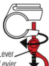
Attach the bracket to the handle bar securely. Place the rubber pad in the bracket to keep the bracket from rattling.
