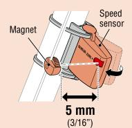
\* The magnet may be mounted at any position on spoke as long as attachment conditions are satisfied.
