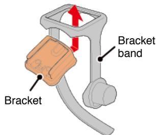
2. Remove the seal from the bracket rubber pad and stick the bracket rubber pad onto the bracket band.
