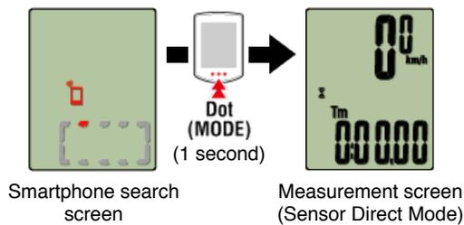
\* Smart computer will search for a sensor instead of your smartphone. In this mode, the sensor icon flashes to indicate sensor reception status.
