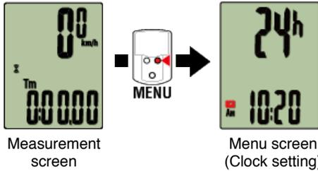
\* When the menu screen is left on for 1 minute, smart computer returns to the measurement screen.
