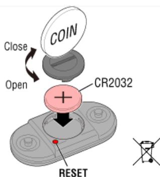
\* After replacing the battery, always press **RESET**.
