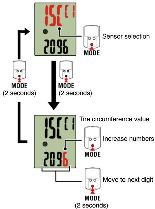
\* Sensors that can be selected are those that have been paired with Cateye Cycling™ or a smart computer. The letter that appears after the sensor name indicates how the sensor was paired.
