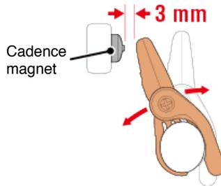
(2) Rotate the sensor arm so that the gap between the wheel magnet and the speed sensor zone is approximately 3 mm, then tighten the sensor screw securely.
