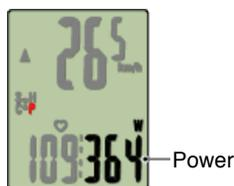
\* When the power value exceeds 999, the last three digits are displayed.
