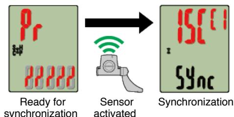
The synchronized sensor is displayed on the top of the screen and pairing is completed.
