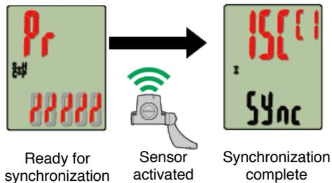
The synchronized sensor is displayed on the top of the screen and pairing is completed.
