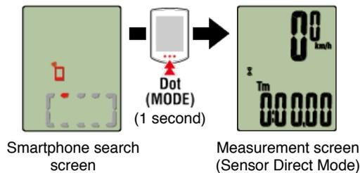
\* Smart computer will search for a sensor instead of your smartphone. In this mode, the sensor icon flashes to indicate sensor reception status.
