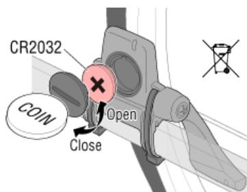
\* After replacing the battery, always press **RESET** and check the position of the sensor relative to the magnet.
