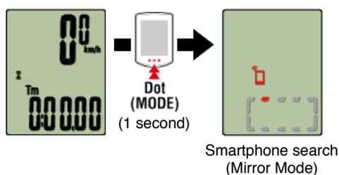
Confirm the change from smartphone search to the connection screen, and the return to the measurement screen.
