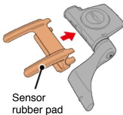
(3) Refer to the illustration and temporarily attach the sensor to the left chain stay with nylon ties.
