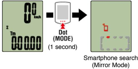
Confirm the change from smartphone search to the connection screen, and the return to the measurement screen.
