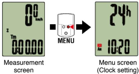
\* When the menu screen is left on for 1 minute, smart computer returns to the measurement screen.
