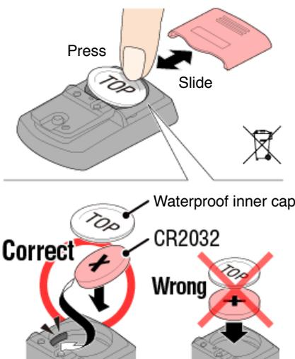
\* Press the top edge of waterproof inner cap to remove it. Install the cap with the "TOP" faced upward.
