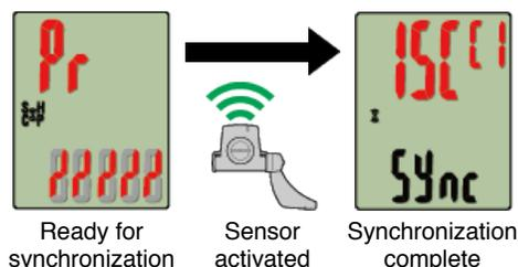
The synchronized sensor is displayed on the top of the screen and pairing is completed.
