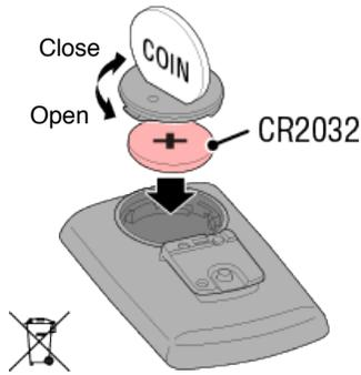
\* After replacing the battery, press **AC** on the back of the computer.
