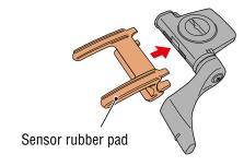
(3) Refer to the illustration and temporarily attach the sensor to the left chain stay with nylon ties.
