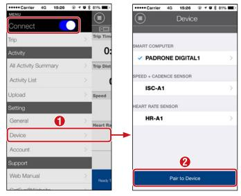
After tapping [Pair to Device], activate the added sensor using the procedure in the following table.
