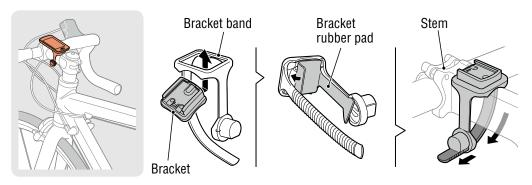
• When mounting on handlebar
