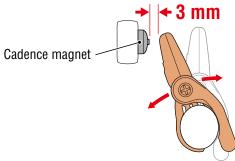
(2) Rotate the sensor arm so that the gap between the wheel magnet and the speed sensor zone is approximately 3 mm, then tighten the sensor screw securely.
