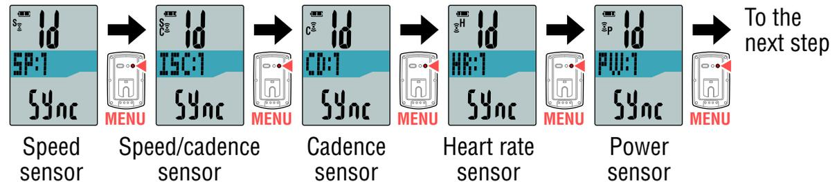
Pressing the **MENU** button with “PW” (Power sensor) goes to the next step. The screen of the next step differs depending on the speed sensor you have searched.
