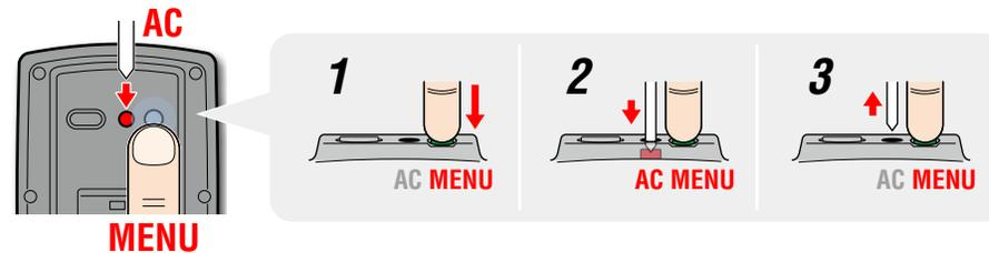
\* Press and hold the **MENU** button for 3 seconds after releasing the **AC** button.
