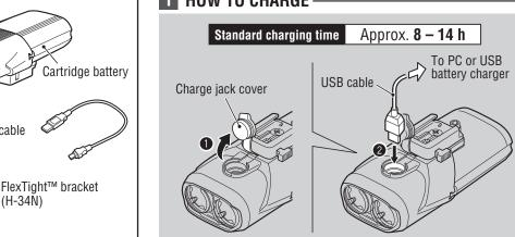
1. Connect the light unit to your PC or a commercial USB battery charger using the USB cable. (Fig 1 (1 - 2)). The switch lights up, and charging starts.
