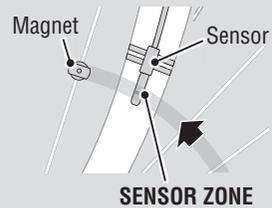
**B** The clearance between the sensor and magnet is 5 mm or less.
