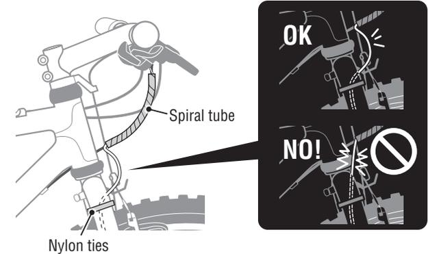
Secure the cord on the fork with the nylon ties and lead to the handle bar along the outer cable of the bicycle by means of the spiral tube.
