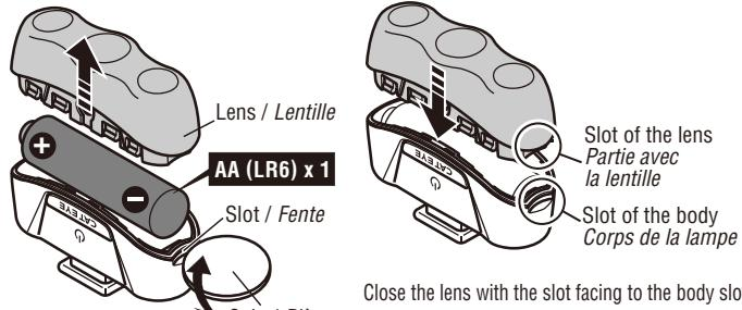
Close the lens with the slot facing to the body slot.
