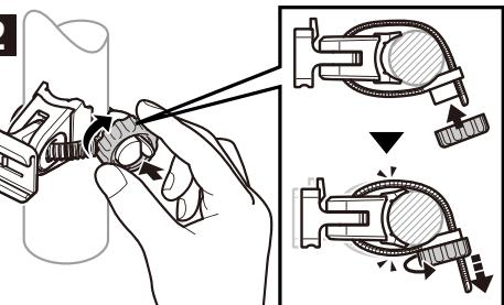
When cutting off the protruding part of the bracket band, rounding the edges to prevent injury.
