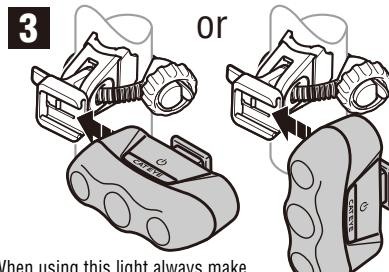
When using this light always make sure to slide the light onto the bracket completely (until it "clicks" into place).
