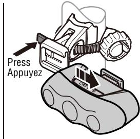
To remove the light, press the lever and slide it off.
