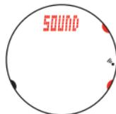
3. Select “**ON**” or “**OFF**” of the button operation sound pressing the **MODE1** or **MODE2** button.
