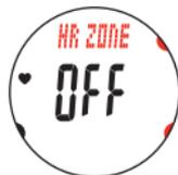
3. Select the target heart rate zone. Select one of "OFF", "ZONE-1", "2", "3", "4" or "5" pressing the **MODE1** or **MODE2** buttons. To set the target heart rate zone, select from "1" to "5" and confirm it pressing the **SSS** button, and then proceed to the step 4. Otherwise, select "OFF" and proceed to step 6.
