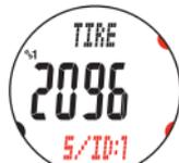
3. Enter the last 2 digits of the tire circumference by pressing the **MODE1** or **MODE2** button, and move digits by pressing the **SSS** button. Then enter the first 2 digits in the same way.
