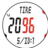
4. Pressing the **MENU** button confirms the tire circumference, and returns to the Setup mode “**TIRE**”.
