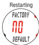
\* Select **"YES"** by pressing the **MODE1** or **MODE2** button for the formatting operation. As the formatting operation deletes all data, select **"NO"** for the restarting operation. See "Formatting/Restarting operation" on page 20 for differences between the formatting and restarting operations.
