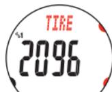
2. When **S1** and “**S/ID:1**” are flashing, confirm with the **SSS** button. Change the tire circumference of Sensor 1.
