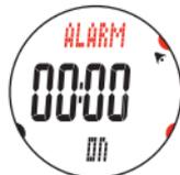
3. Select **"ON"** or **"OFF"** pressing the **MODE1** or **MODE2** button. To use the alarm clock, select **"ON"** and press the **SSS** button to proceed to Step 4. Otherwise, select **"OFF"** to proceed to Step 5.
