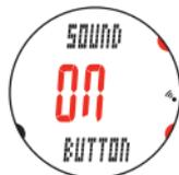
4. Select “**ON**” or “**OFF**” of the target heart rate zone alarm sound pressing the **MODE1** or **MODE2** button.
