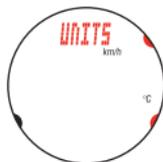
2. Select the speed unit by pressing the **MODE1** or **MODE2** button, and confirm with the **SSS** button.
