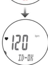
\* This unit enters the search mode for 5 minutes after starting the ID sync. Press the **SSS** button in the search mode to cancel the ID synchron, and “**ID-SKIP**” is displayed. If any sensor signal is not received in 5 minutes, “**ID-ERROR**” is displayed. When “**ID-SKIP**” or “**ID-ERROR**” is displayed, the ID has not been synchronized properly.
