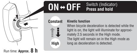
When the remaining battery power is low, the lighting mode switch turns on. Charge the light as soon as possible.
