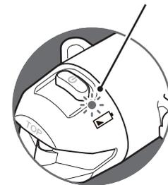
**⚠ Install the unit with the switch facing up.**
