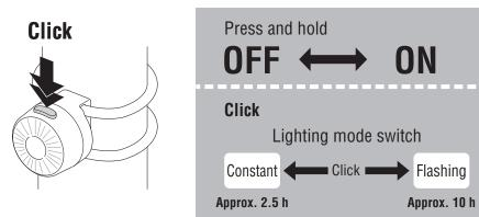
\* When the remaining battery power is low, the indicator beside the switch turns on. Charge the product as soon as possible.
