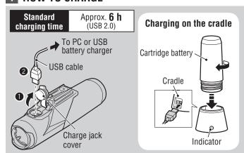
Connect the light unit to your PC or a commercial USB battery charger using the USB cable. (Fig 1 1 - 2)
