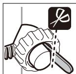
When cutting off the protruding part of the bracket band, round off the edges to prevent injury.
