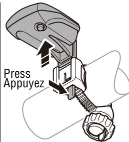
When using this light always make sure to slide the light onto the bracket completely (until it "clicks" into place).
