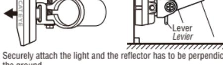
Securely attach the light and the reflector has to be perpendicular to the ground.
