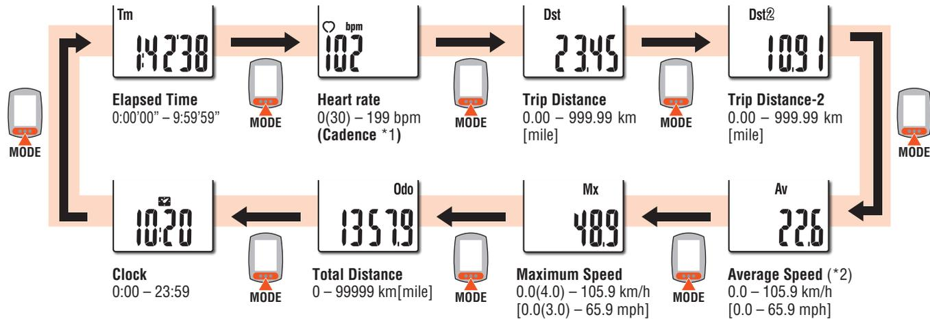
\*1 In combination with the optional speed sensor (ISC-10), it displays the cadence.
