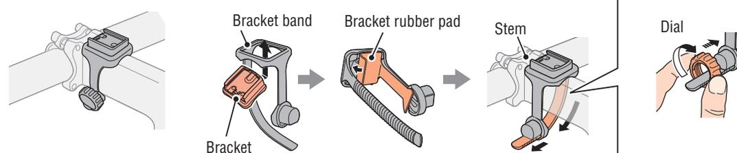
When attaching the FlexTight™ bracket to the handlebar :
