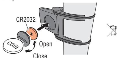
\* After replacement, check the position in respect to the magnet.
