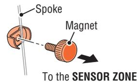
\* The magnet may be installed anywhere on the spoke if the above installation conditions are satisfied.
