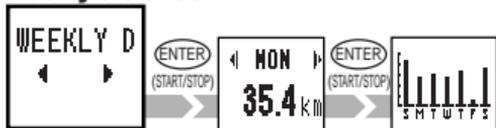
A week's trip distance is displayed day by day. Press ENTER/START/STOP button and the screen shows the data in the graph format. (Maximum value of the graph: 120km, Minimum value of the graph: 5km)
