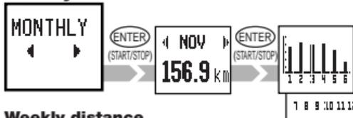
The monthly distance is displayed for one year. Press ENTER/START/STOP button and the screen shows the data in the graph format by six months period. (Maximum value of the graph: 1200km, Minimum value of the graph: 50km)
