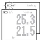
If this indicator appears, the battery is beginning to run down. When the battery is consumed further, it begins to flash.
