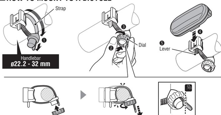
1. Attach the bracket to the handlebar as shown in the drawing. (1 - 3)
