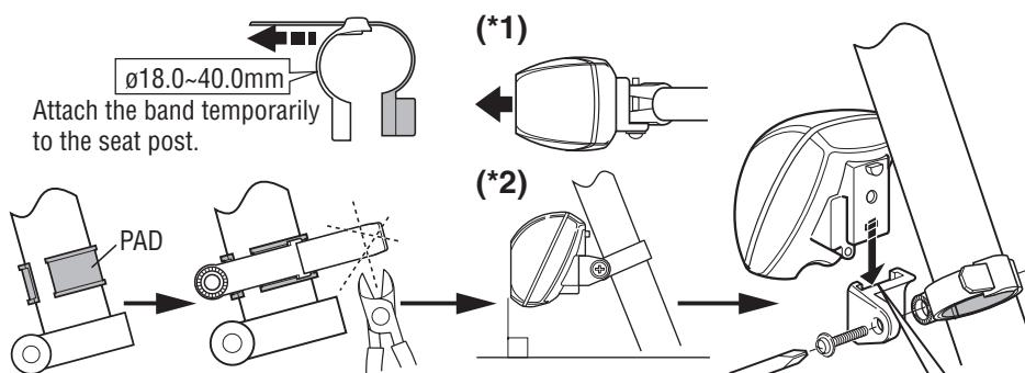
1. Install the rubber pad on the clamp as shown and attach it to the seat post.
