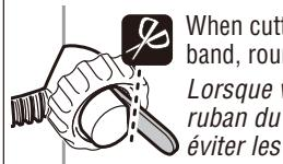
When cutting off the protruding part of the bracket band, round off the edges to prevent injury.
