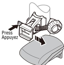
When using this light always make sure to slide the light onto the bracket completely (until it "clicks" into place).
