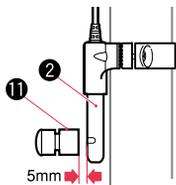
Speed Sensor and Wheel Magnet
