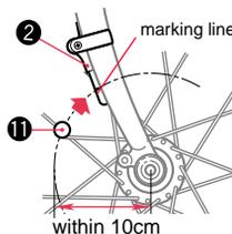
Speed Sensor and Wheel Magnet
