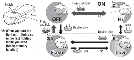
\* When the switch (indicator) lights up, the remaining battery power is 20% or less. Please charge as soon as possible.
