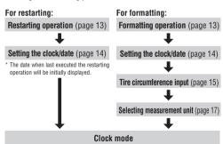
\* In the case of the formatting operation, you can set the "tire circumference" and "measurement unit" sequentially after you set the "clock/date". Each set-up procedure is described on the page referenced.
