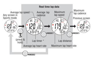
\* Press the MODE2 button with the real time lap data to return to the previous Sports mode screen.
