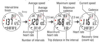
Press the LAP button to start the next repeat of the interval time again. Start pedaling at your interval intensity. Repeat the steps 4 and 5.
