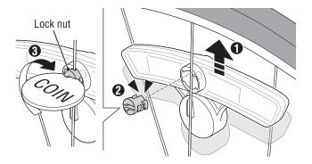
Place the nut into the reflector hole putting the spoke in between then tighten it securely using a coin.
