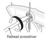
To remove the reflector, insert a flathead screwdriver into the lock nut, and then turn the lock nut in the counterclockwise direction.
