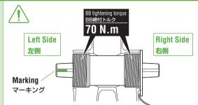
When installing the BB, be especially careful not to damage the cable from the BB. When tightening the BB,
